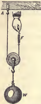
FIG. 46.—The Effort F Equals One Half of the Weight W , but Moves Twice as Far.
